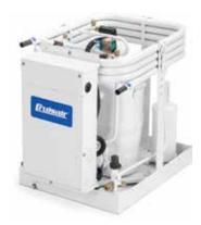
Available in capacities from 20,000 to 48,000 BTU/hr, Type R remote condensing units represent the next generation of seawater-cooled, reverse-cycle heat pumps for cooling and heating in marine applications. Models up to 36,000 BTU/hr use reciprocating compressors, while the 48K units use scroll compressors.
